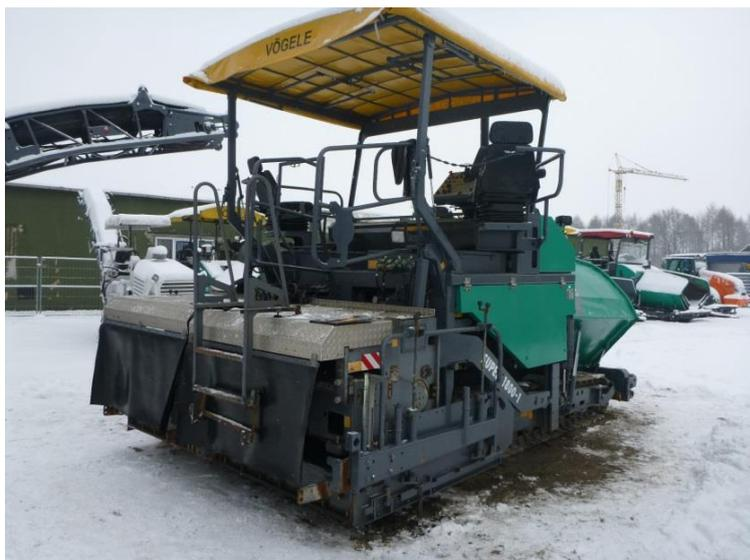
The inspection starts with a configuration check. Serial numbers and chassis number will be approved. The inspector then does a visual walk-around check for cracks, leaks and damage etc. This is then followed by an operational test of all systems such as the hydraulic system along with testing of the drive train. Depending on possibility we also check the screed and the screed heating system.
